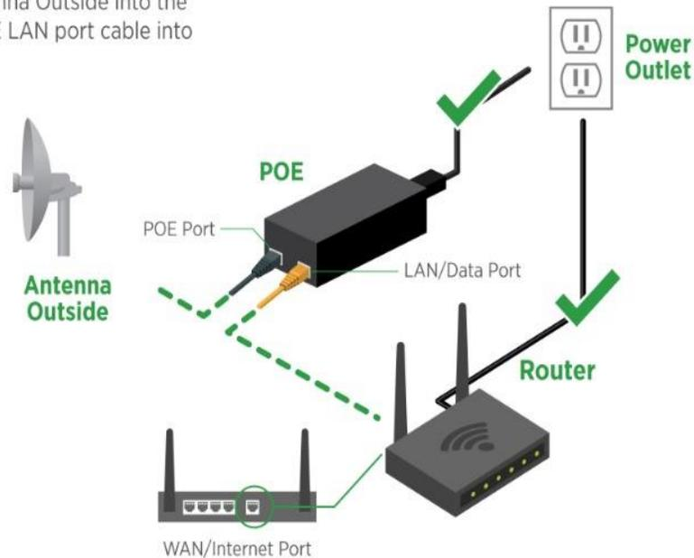
If you want to connect multiple devices to the internet through a wired or wireless connection, you'll need a router. You can set your router up right along with your POE. Instead of plugging the POE directly into your computer, you'll plug it into the router with an Ethernet cable. After that, you'll take a second Ethernet cable and connect the router to your computer. In essence, you're linking your computer to the modem *through* the router.
